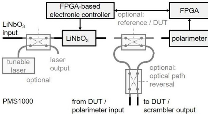
PMS1000 for measurement of Mueller and Jones matrices and PMD of a device under test (DUT). Optional components are shaded. C&L band tunable laser modules are available (usually in LU1000 laser unit). EPS1000 polarization scrambler/transformer and PM1000 polarimeter are individually accessible, even when they are combined into one unit.
