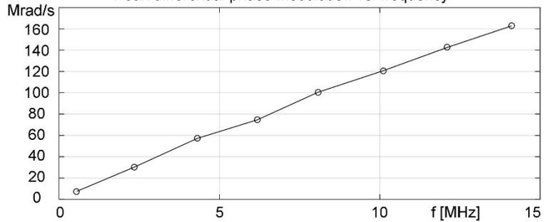
A LiNbO<sub>3</sub> phase modulator is investigated as another DUT. From the measured time-resolved Mueller matrices the differential phase modulation is extracted (peak value: 163 Mrad/s).
