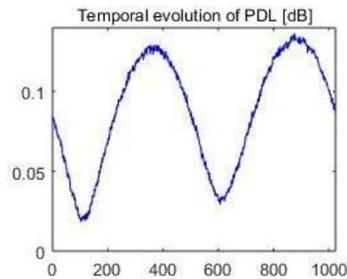
Time-resolved PDL of a rotating electrooptic halfwave plate (EPS1000) as a DUT, extracted from 1024 Mueller matrices recorded with **320 ns** temporal spacing.
