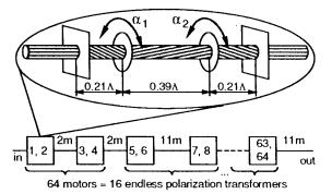
Fig. 13. Distributed PMD equalizer with PMF twisters.
