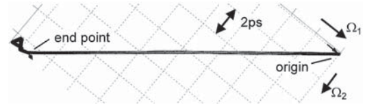
Fig. 14. DGD profile of one 25-ps DGD section. The \Omega_3 component is not seen in this projection.
